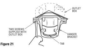
**2.** Carefully lift the fan and seat the hanger ball/downrod assembly on the hanger bracket that was just attached to the outlet box (Figure 22). Be sure the groove in the ball is lined up with tab on the hanger bracket (Figure 21).
